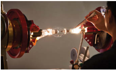
Lamp sealing process. The electrode assemblies are inserted into the lamp envelope and the quartz material is fused together to provide a strong, gas-tight seal.
