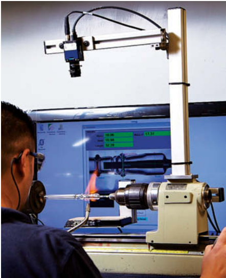
Building lamp seal assembly. Multiple layers of glass with different expansion coefficients are built up under vision system guidance, to allow the seal to compensate for the difference in expansion rates between quartz and tungsten.
