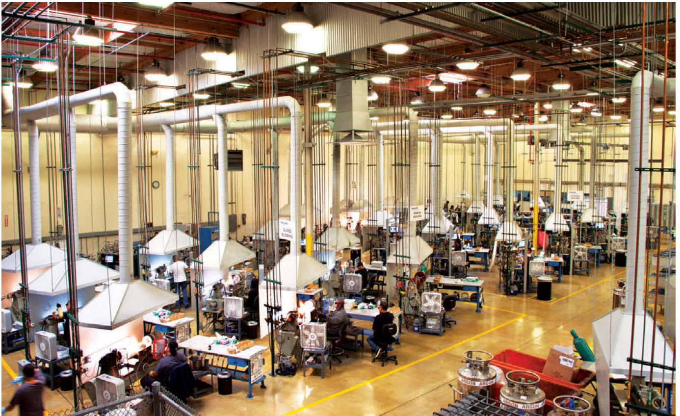
Just part of the massive manufacturing and production area. Notice the multiple workstations with extensive fume extraction equipment and ducting, used to remove the heat from the glassworking operations, always ensuring that the atmosphere is clean, safe, and comfortable for the operators to work in.
