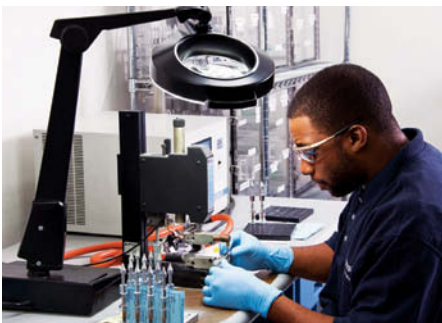
In another part of the factory Electrode assemblies being spot welded. These assemblies are put together by hand to exact specification.
