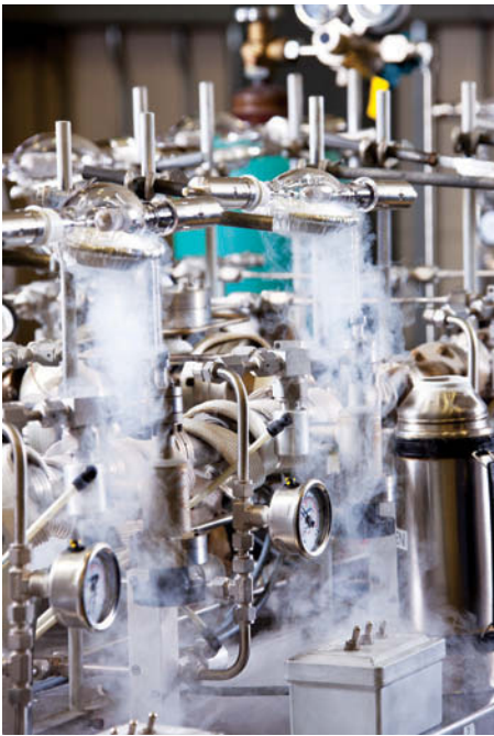
Close up of lamp xenon gas filling process.
