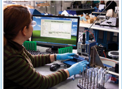
The thickness of the electrode glass seal assemblies are 100% inspected using a high accuracy digital microscope, to ensure all assemblies are built within specification.
