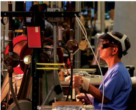
Operator sealing a xenon lamp. Most lamp manufacturing operations are performed on specialized glassworking lathes.
